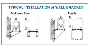
NOTE: It is the manufacturer's recommendation that the racket be used fo wall mount applications. Contact the factory concerning other mounting considerations. Sometimes are factory concerning other mounting considerations. It is also recommended that suction lift be kept to a minimum and should be a consideration in choosing shelf mount loca-
