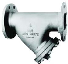
Fig. #381(Flanged) 125# WSP 200# WOG "Y" Strainer Bolted Cover, SS Screen
