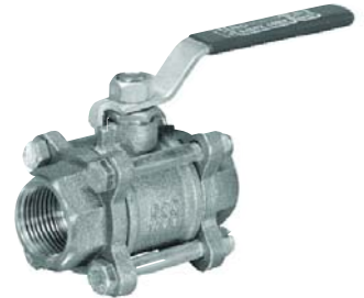
Fig. #5050 & #5051 #5050-Threaded Ends #5051-Solder Ends 150# WSP 600# WOG 3-Piece Full Port Chromium-Plated Ball Teflon Seats, Blow-Out Proof Stem
