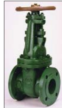
F-637-33-Solid Wedge sizes 2" to 4" inches Flanged-Raised Face
