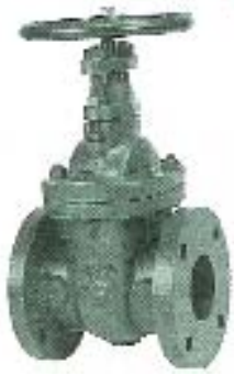
Fig. 619-Gate 2 to 12 inches Inside Screw Non-Rising Bronze Stem Renewable Bronze Seats and Disc
