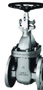
Fig. #415(Flanged) 125# WSP 200# WOG Gate Valve IBBM, NRS Solid Disc MSS-SP-70
