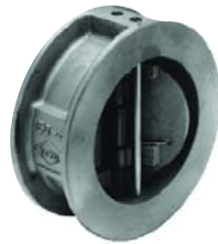
Fig. #442(Flanged) 150# WOG Dual Plate Check Valve Bronze Plate Buna-N Seat
