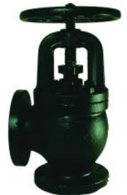
Iron-Bronze Mounted Fig. F-869-B-Angle 3 to 8 inches 450°F. 250 lb. S.P.
